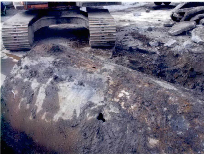
Photo 9: The upper half of the USTs were observed to be highly corroded and pitted, with holes up to several centimeters in size.
