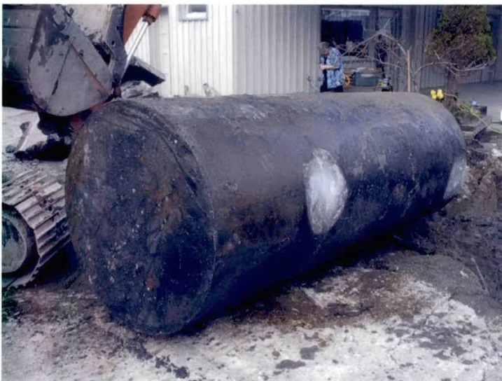
Photo 8: The lower half of the tanks (except UST #4) were observed to be in good condition, with only minor corrosion and pitting and no holes. The lower half of UST #4 was highly corroded and had holes.
