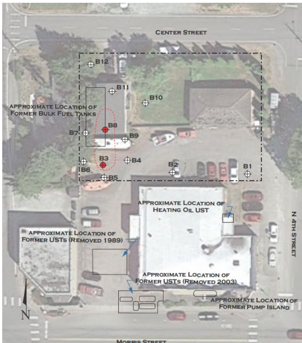
Figure 1: This photo shows the 12 boring sites where soil samples were taken in 2022 and 2023. The borings marked in red (B3 and B8) indicate contaminants detected in the soil.
