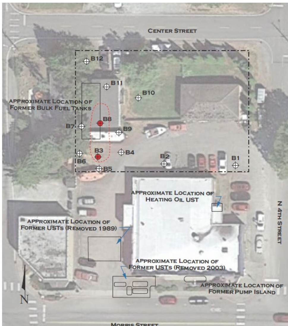
Figure 1: This photo shows the 12 boring sites where soil samples were taken in 2022 and 2023. The borings marked in red (B3 and B8) indicate contaminants detected in the soil.
